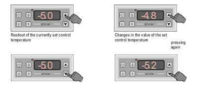
The change of the set control temperature takes place at the moment of automatic exit from the settings and readout of the control temperature.
