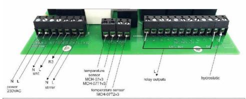
In case of using the washing program with the stirrer control, output of the stirrer L and output R3 can be connected. In this configuration stirrer control will take place both from the cooling segment and the washing segment as well, in accordance with the set program.
