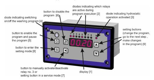
The UMS controller is equipped with:
