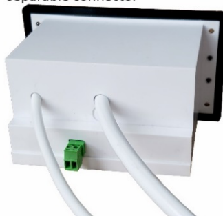
SMT-03 outputting inputs and outputs using screwed connections
