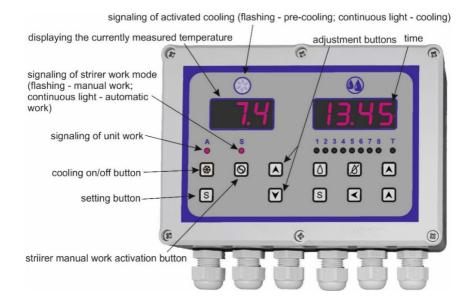
Within approx. 2 min. after connecting the controller to the supply voltage, it is possible to turn on the cooling section and the washing section at the same time. After this time has elapsed, the washing process is blocked during cooling.
