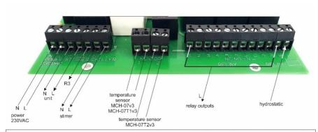
In case of using the washing program with the stirrer control, output of the stirrer L and output R3 can be connected. In this configuration stirrer control will take place both from the cooling segment and the washing segment as well, in accordance with the set program.
